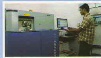
Chemical Composition Testing by Spectrometer
