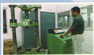
Tensile Strength Test by UTS Machine
