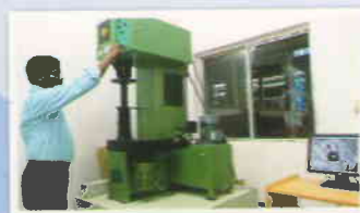
Hardness Testing by Brinell Hardness Testing Machine
